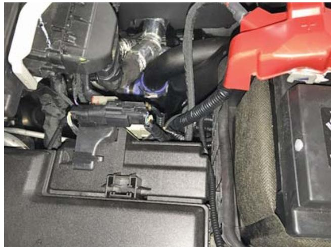
6. Remove one (1) nut with a 10 mm socket from the front positive terminal post. Install the positive ring terminal from the marker light wiring harness (P/N: 1115-15N515) and re-secure the 10 mm nut that was removed. Torque to 8-10 Nm.
