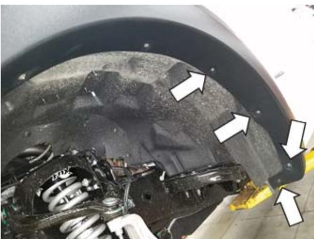
8. Set the rear fender flares in place to mark the locations for the mylar pads. Apply one (1) mylar pad in each of the locations shown below and fold them around the lip of the wheel wells. Install one (1) J-clip around each of the mylar tabs.
