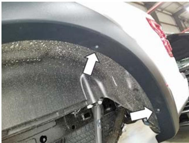
12. Use the supplied nylon trim tool and carefully slide it along the edge seals to ensure that they are fully seated.
