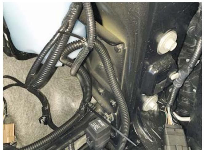
3. Route the two (2) ring terminals and the fuse tap up along the battery box. Secure the fuse plug and harness with the supplied zip ties (P/N: CTUV740) as shown.
