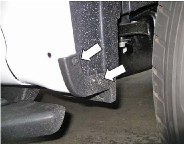
3. Pull firmly outwards on the wheel lip moldings (if equipped) to remove them from the front fenders. Use a non-marring trim tool if needed.
