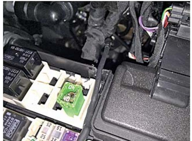
8. Install the 7.5 amp fuse that was previously removed into the fuse tap of the marker light wiring harness (P/N: 1115-15N515). Reinstall the fuse tap into the same location from which the fuse was originally removed. Trim the fuse box to allow clearance for the fuse tap lead and route the fuse tap lead through the trimmed area as shown.
