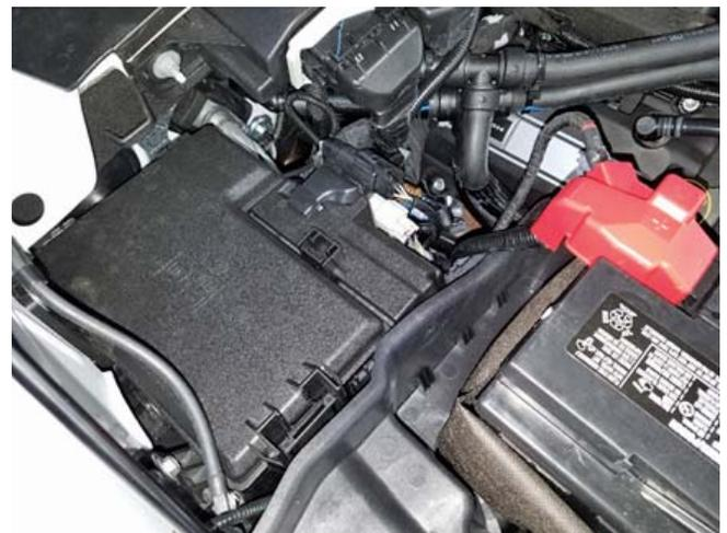
10. Route the wire harness (1115-HWKWHN) along the front core support and secure with the provided zip ties (P/N: CTUV740) as shown.
