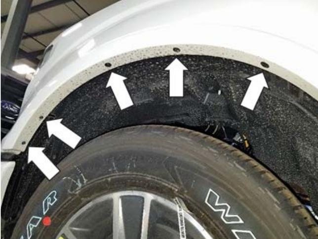
2. Remove two (2) fasteners with a 7 mm socket from the rear of each front wheel well.
