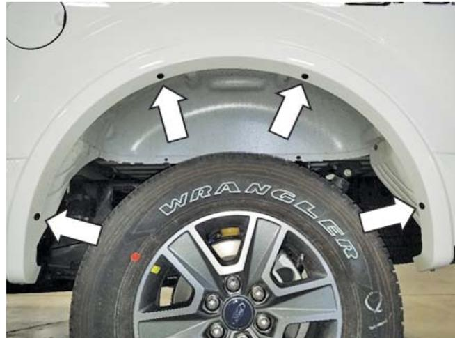
11. Firmly pull outwards on the factory rear wheel well moldings to remove them from the bed sides.
