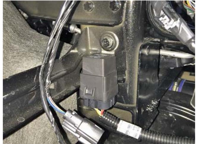
2. Route the two (2) ring terminals and the fuse tap up along the factory harness that passes over the windshield solvent bottle as shown. Secure with the included zip ties (P/N: CTUV740).
