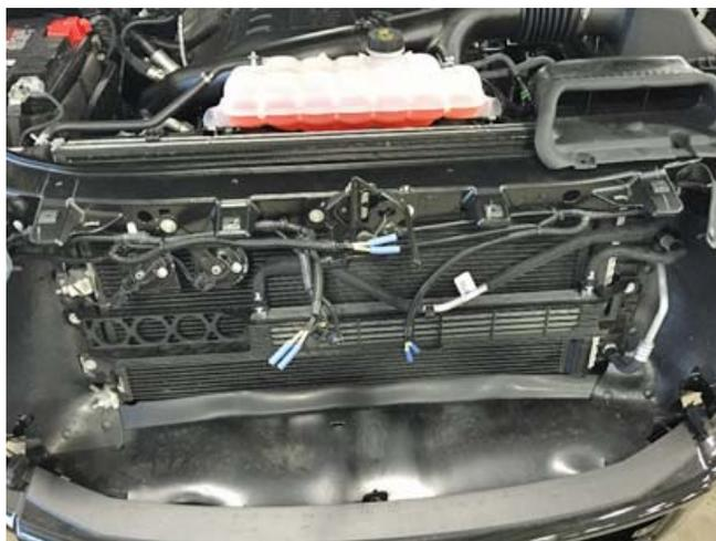
13. Reinstall the headlight, grille and radiator close out panel by following the reverse of steps 6 through 9 in the Disassembly section.
