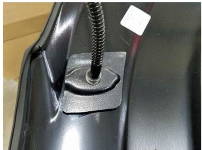
4. Install one (1) red marker light assembly (P/N: 1115-REDLTE) into each of the rear marker light brackets. Remove the red backing from each piece of tape and secure the assembly to each rear fender flare as shown.
