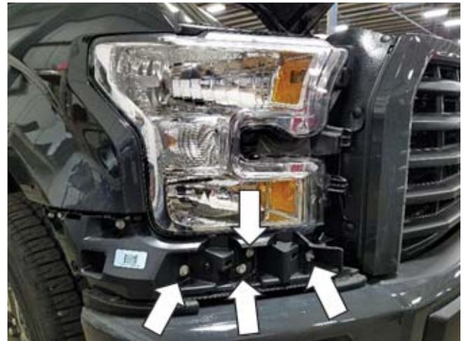
8. Remove two (2) screws with a 10 mm socket which retain the headlight. Disconnect the electrical connectors and set the headlight aside in a safe place.
