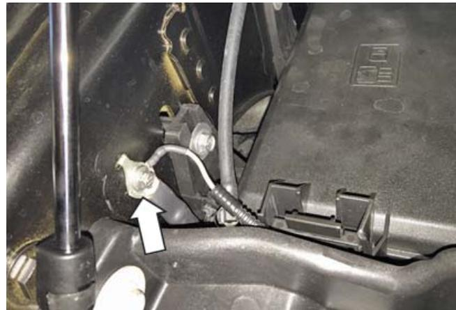
5. Remove the positive terminal cover from the fuse box.
