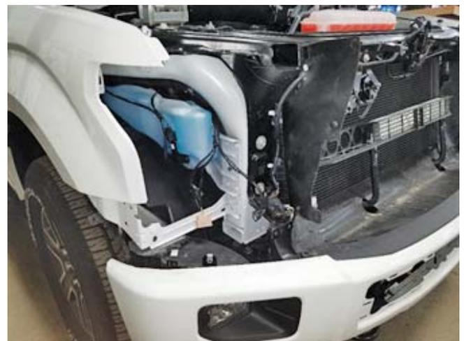
9. Remove three (3) push pins with a trim tool and one (1) screws on each side of the grille with an 8 mm socket. Remove four (4) screws on top of the grille with a 10 mm socket. Disconnect the electrical connectors and remove the front grille assembly.
