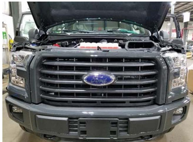
11. Securely fasten the three (3) sets of connectors for auxiliary grille lighting and ensure that none of the wiring will be pinched when re-installing the front end components. **NOTE:** If desired, these connectors can be used to install additional 12-volt lighting. However, Roush Performance is not responsible for any problems that may occur as a result of improper installation of any auxiliary lighting that is not supported by Roush Performance.
