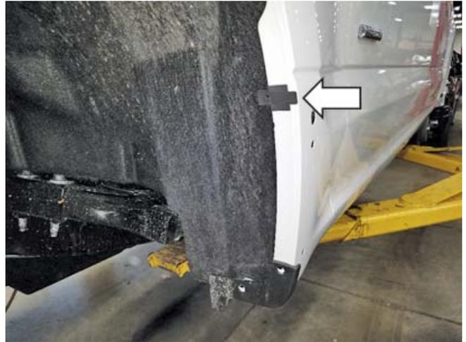
3. Install one (1) front fender flare inner retaining bracket on each side of the vehicle using the three (3) screws that were removed in the previous step. Torque to 0.9-1.1 Nm.
