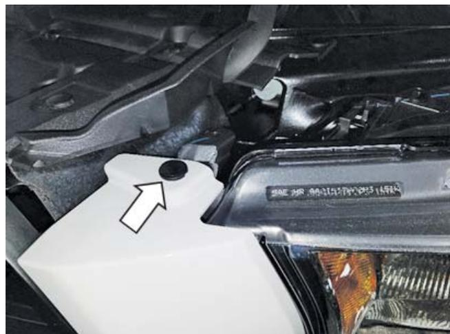
6. Remove nine (9) push pins and set the radiator close out panel aside.
